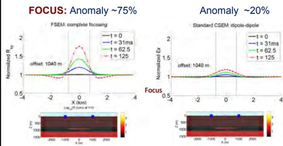
Figure 3: Focussed EM modeling example for a hydrocarbon reservoir (left) and the corresponding anomaly from a standard TEM survey.
