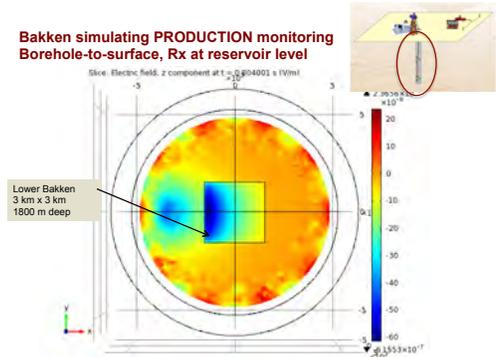
Figure 3: Simulation snapshot of electric field values measured downhole in a shale reservoir. The blue and the red colors are high and low current densities.
