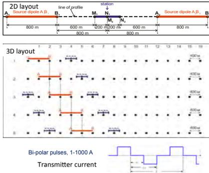
Figure 2: Focussed EM layout for 2-D and 3-D land acquisitions. The source wave form is shown at the bottom. Examples transmitter and receivers are shown in Figure 1.
