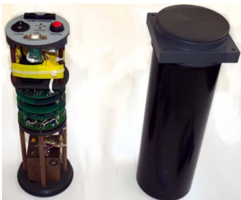
Fig. 3. External view of LEMI-026 magnetometer both with weather-proof housing (left) and without it (right).
