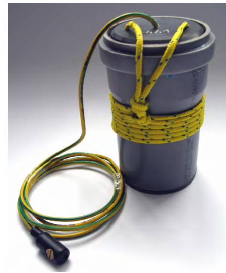
Figure 1: LEMI-701 ultra-low noise non-polarized electrodes.
