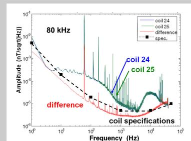
Fig. 4: Parallel test with HF coil Lemi-118
