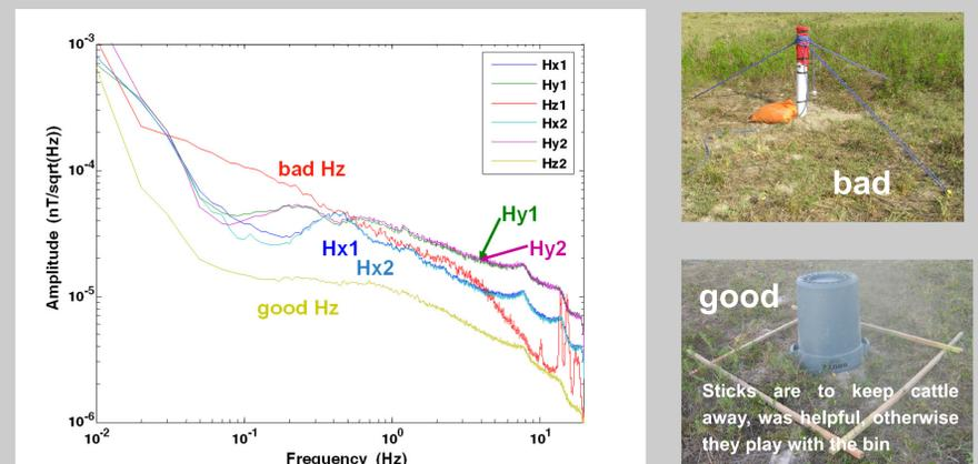
Fig. 6: Parallel set up of 2 MT stations, all magnetic fields recorded with 40 Hz sampling are shown. The good Hz is smaller in amplitudes as horizontal components and the bad solution in spite of a tube and trial of fixing it is out of order in the whole frequency range.
