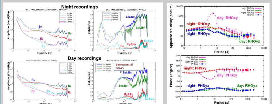
Fig. 11: Spectra (left), coherence (middle) and apparent resistivity & phase (right for night (top) and day (bottom) recording).
