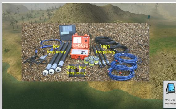
Fig. 1: Equipment of one MT station.
