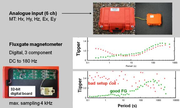
Fig. 7: 3C digital fluxgate magnetometer with specifications and 2 examples of tipper recorded in good terrain conditions for the vertical induction coil and for a bad setup.
