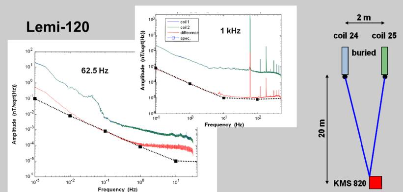
Fig. 5: Parallel test with LF coils Lemi-120 for low 62.5 Hz and high 1 kHz sampling rate
