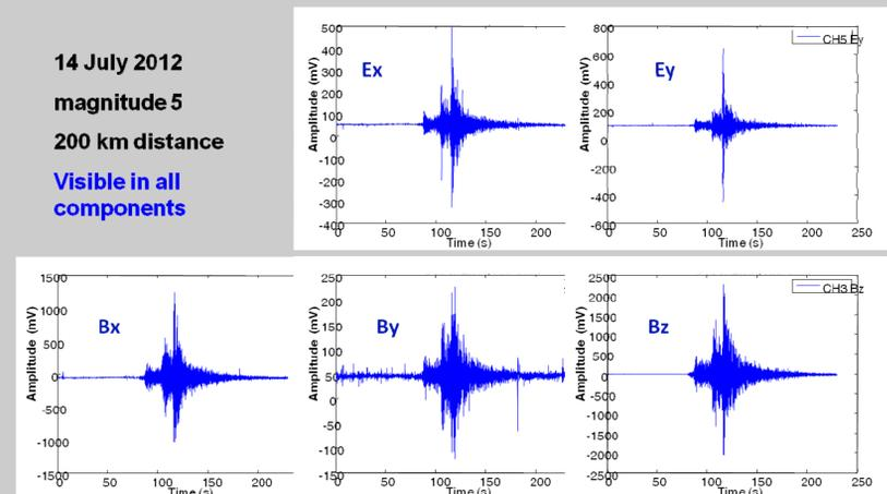
Fig. 10: Amplitude of electric and magnetic fields for all 5 components as function of time
