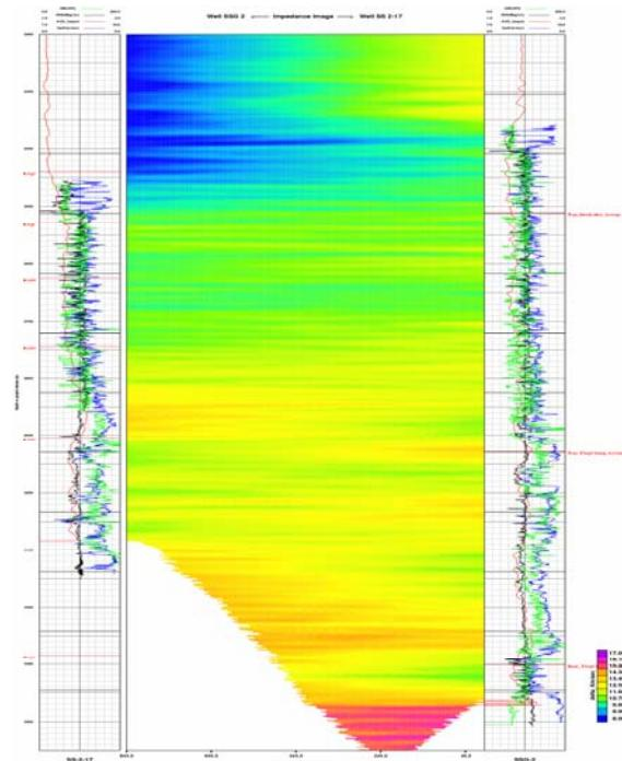
Figure 3: Final AVA-Vp inverted acoustic impedance image.
