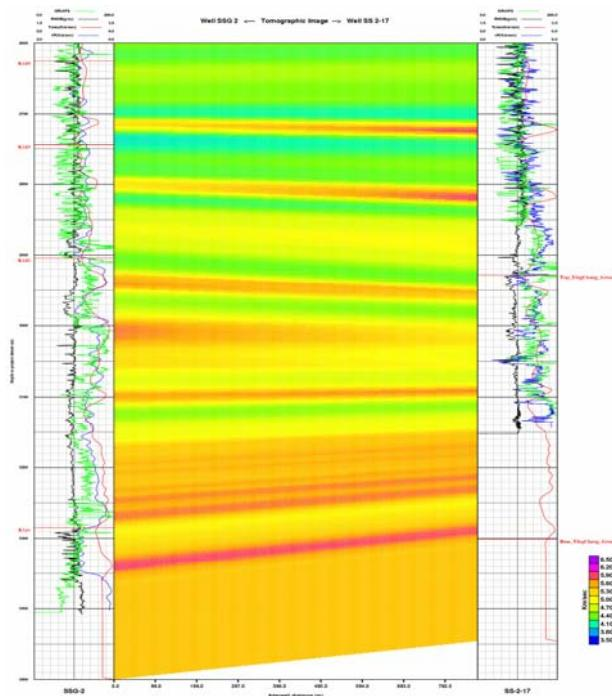
Figure 1: Final tomographic inverted velocity model.
