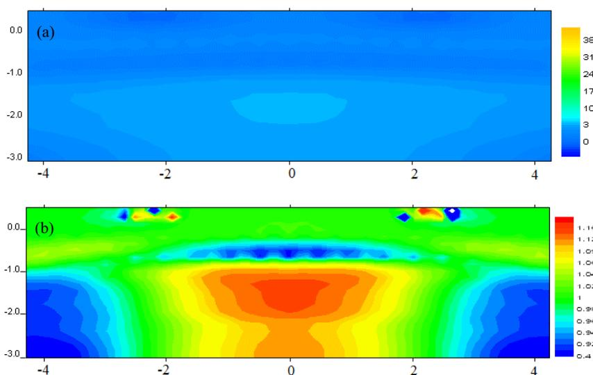
Figure 8: (a) Apparent resistivity profile (b) Generalized resistivity profile.
