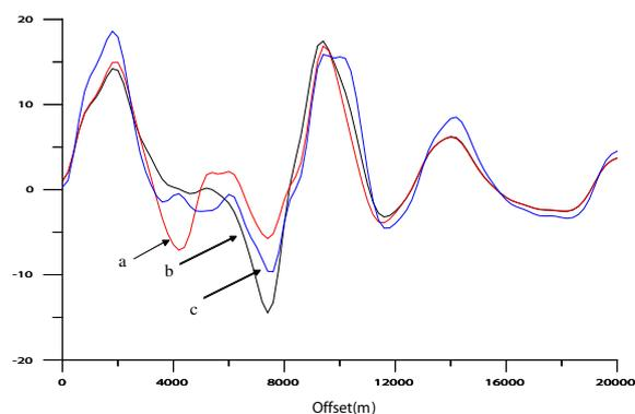
Figure 7: MVOSD curves for a model composing three resistive bodies Vertically. a. The upper resistive body is 4 km wide, the lower 7 km wide, b. The upper resistive body is 7 km wide, the lower 4 km wide, c. The upper resistive body is 3 km wide, the middle 5 km wide.
