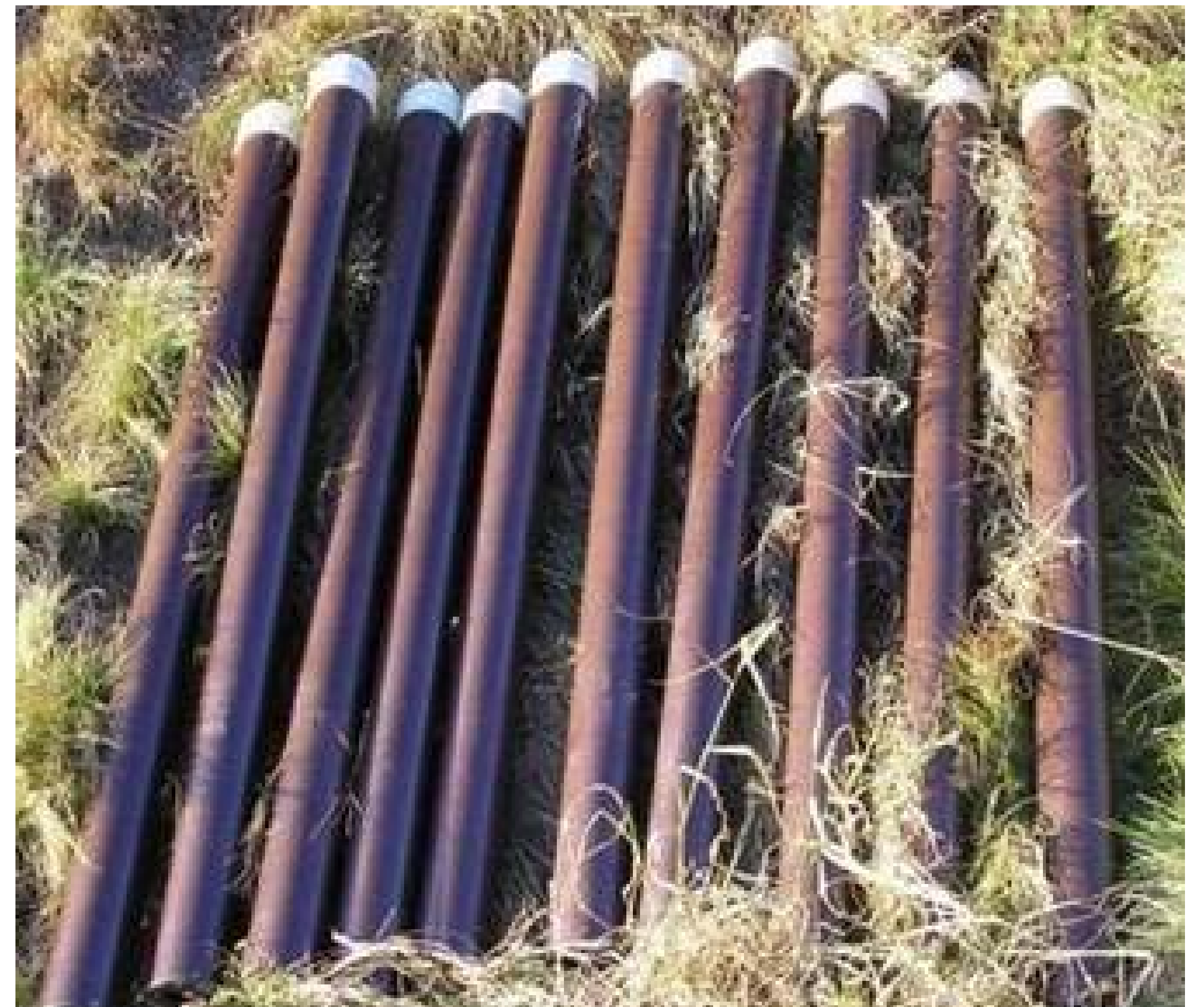
LEMI-120 land induction coil magnetometer
