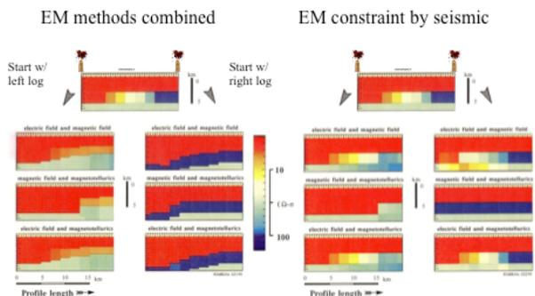
**Figure 4. Inversion examples using various electromagnetic methods. On the left side the synthetic data was inverted unconstrained and on the right side, the data was constrained with seismic. (after Strack et al., 1989).**
