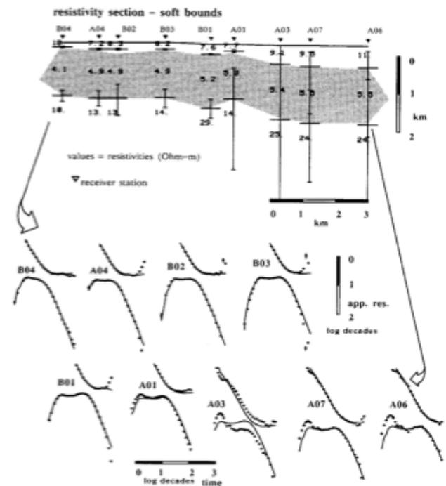
**Figure 6. Resistivity inversion results using constrained inversion. Here the inversion bounds on one side are linked to the neighbouring sites (after Strack et al., 1989).**
