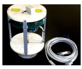
needs of fundamental and applied geophysics. It has no external housing being destined for the installation inside sealed housing of sea bed station (see photo on the left). Because of this any customization of dimensions are possible at the customer's request. It has twocomponent tiltmeter and does not contain GPS receiver and nonvolatile memory. For data registration it has to be coupled with a basic station by a cable
