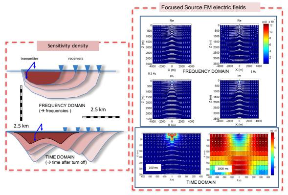
Figure 3: Sensitivity plots for frequency and time domain CSEM on the left and on the right for FSEM.
