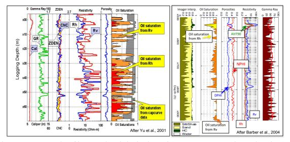
Figure 2: Two examples of interpreted 3D induction logs using 3-component transmitter and receivers. In both cases the improved oil saturation is shown in the orange shaded track.
