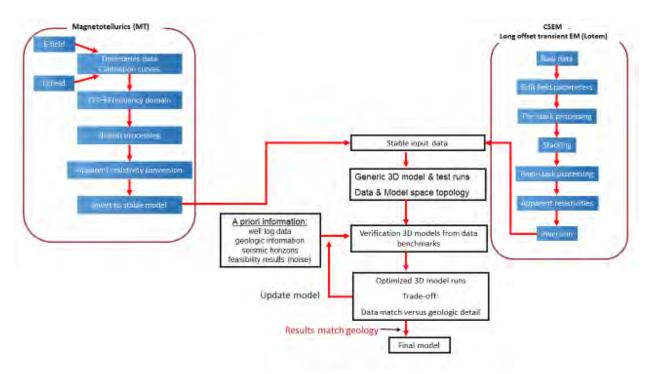
Figure 2: A schematic diagram of various processing workflows including processing and interpretation to final 3D model.
