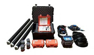
Figure 1: The main components of the array system: 1) KMS-820 digital acquisition system, 2) LEMI-120 low frequency magnetometer, 3) LEMI-701 electrodes, 4) KMS-831 sub-acquisition controller, 5) KMS-029 fluxgate magnetometer, 6) KMS-410 lithium ion battery, and 7) miscellaneous connection cable
