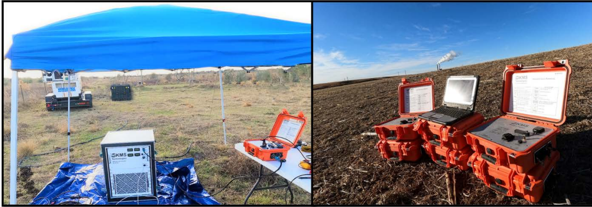
Figure 2: Left: CSEM high-power transmitter, up to 400 Amps reversing (KMS-150). Right: EM receivers (KMS-820 array system). The same receivers are used to record MT/AMT and/or CSEM.
