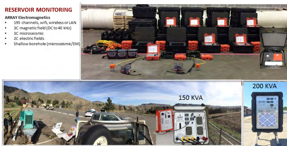
Figure 1- Field equipment and hardware components. Orange boxes: 195-channel microseismic-EM receivers KMS-820.
