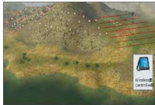
Fig. 4: Seismic-style layout example of an electromagnetic survey using wireless nodes in a regular grid layout and also in irregular lines.
