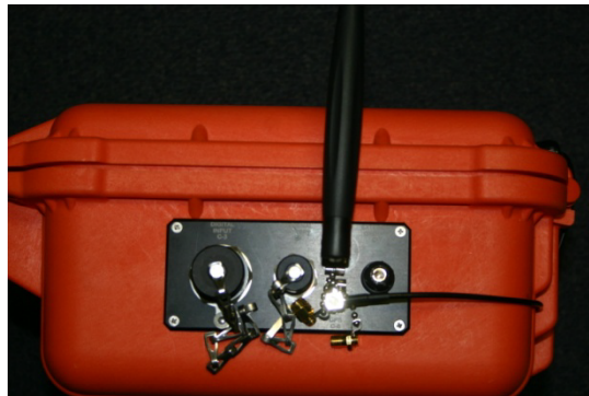
Figure 14 - 900 MHz to 3dBi wireless antenna and GPS antenna installed on the KMS-820
