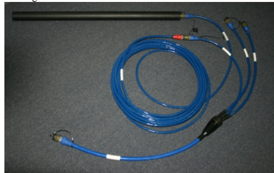
Figure 8- LEMI-118 connected to KMS-105 then KMS-100
