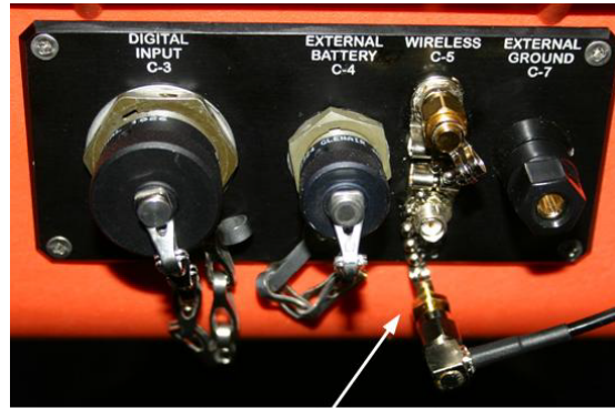
Dust cap installed to on-board GPS cable Figure 16 - GPS dust cap installed
