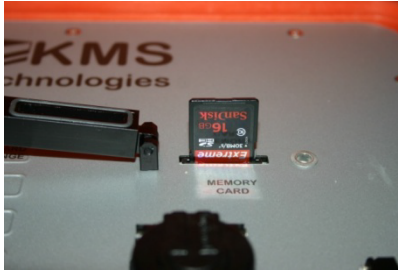
Figure 19 - SD card installation
