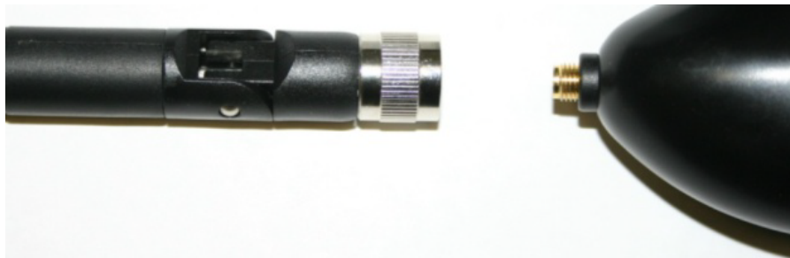
Figure 18 - 900 MHz wireless antenna to KMS-120
