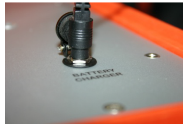
Figure 21 - Battery charger connected to the KMS-820
