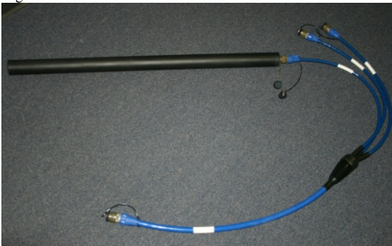
Figure 7 - LEMI-118 directly connected to KMS-100
