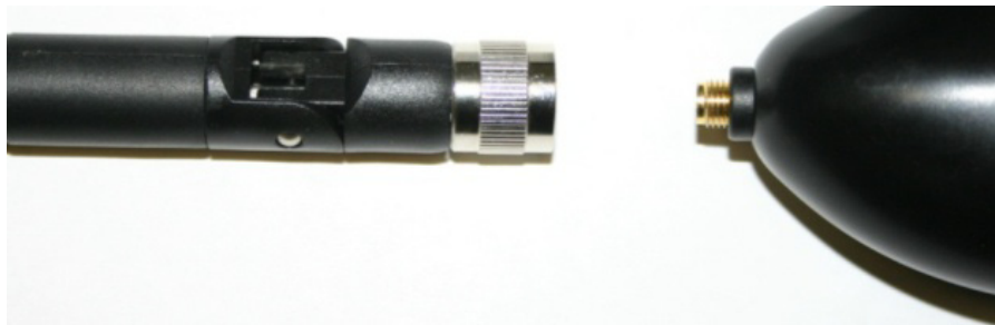
Figure 18 - 900 MHz wireless antenna to KMS-120
