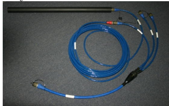
Figure 8- LEMI-118 connected to KMS-105 then KMS-100
