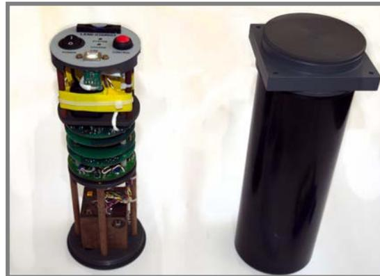
Figure 1: LEMI-026 system with and without housing cover.
